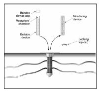
**1b.** Remove termites from the monitoring device into the collecting pan and introduce them into the top of the Baitube.
